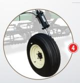
Optional Wing Wheels Optional wing wheels utilize phasing cylinders that allow the unit to lift and lower evenly.
