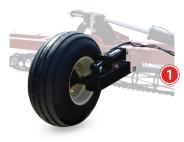
Wing Wheels Our wing wheels utilize phasing cylinders that allow the unit to lift and lower evenly.
