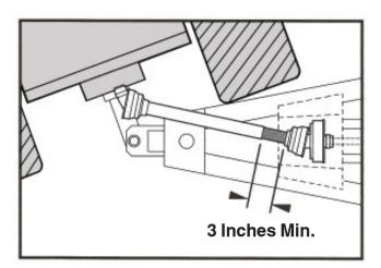
Position the tractor and grain cart to obtain the tightest turning radius. Connect the PTO to the tractor. Be sure the PTO is extended at least 3 inches.
