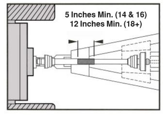
Connect the PTO shaft to the tractor. Measure the PTO overlap length. To prevent uncoupling, make sure there is at least 5 inches of PTO overlap for 14 and 16 inch diameter augers or 12 inches of PTO overlap for augers 18 inches and larger.
