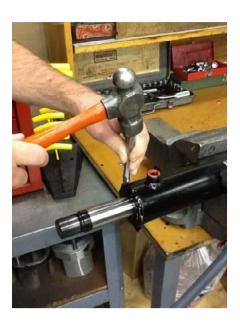
Using a rubber mallet and flat punch, carefully tap the gland into the barrel until it is just past the retaining ring, exposing it. Remove the retaining ring.
