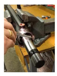
Pull the rod straight out of the barrel removing the gland and piston with the rod.
