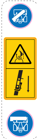
When Moving Auger Tube from Storage Position to Field Position, Ensure Auger Rest is in Field Position. Damage to the Tube Can Occur if Auger Rest is in Storage Position During the Process.
