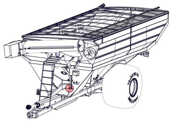
Remove the 1/2" and 1/4" hydraulic hoses from the tank.
