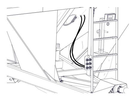
Connect the hoses removed in the last step to the hydraulic block.
