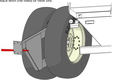
Swing the walker frame weldment back into place. It will have a stop welded inside shown in red in the image.
