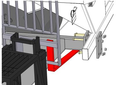
If your cart is set up in the outside hole you should mark where your plates will line up in the back of the cart.
