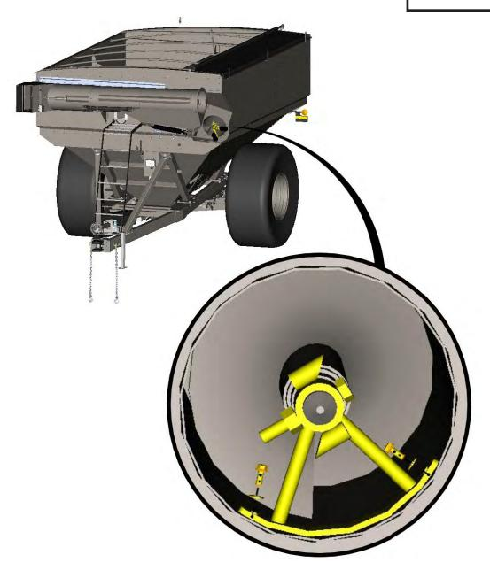
Unbolt the Hanger Bushing Assembly. Use a 9/16" wrench to remove the 3/8" x 1-1/4" hex head bolts. Keep the 3/8" bolts and washers, they will be used in a later step.
