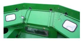
**Step 3** Attach the four rounded corner tip up panels to the tabs on the ends of the corner tip up panels and secure using lynch pins.
