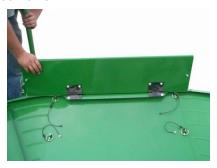
Step 2 Connect the front and rear tip up panels to the tabs located on each end of the tip up corner panel and secure using lynch pins. Center and adjust the panels as necessary. Align the hinges on the front and rear tip up panels with the top edge of the existing tank panels. Drill 3/8" holes at each hinge hole location and secure to the existing tank front and rear panels using 5/16" x 5/8" bolts and 5/16" lock nuts. Tighten all the bolts on the tip up panel hinges.
