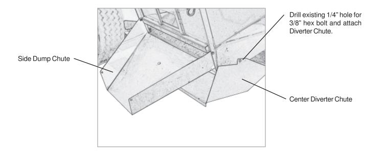
2. Lift the Side Dump Chute up into storage position. Rotate the Center Diverter Chute up against the Side Dump Chute. Extend the chain on the Center Diverter Chute up to the center of the Side Dump Chute so the chain is tight. Mark and drill one 3/8" hole in the Side Dump Chute and attach the chain a couple of links from the end using one 3/8" stove bolt and nut. Be sure to position the head of the stove bolt on the inside of the Side Dump Chute.
