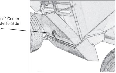
Attach chain of Center Diverter Chute to Side Dump Chute
