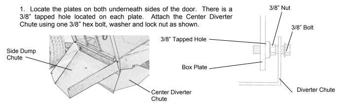
Insert the 3/8" bolt through the pre-punched hole in the chute. Thread the nut onto the bolt until approximately half of the threads are exposed. Screw the bolt through the pre-tapped hole in the plate under the gravity box until the nut is against the plate. This allows the bolt to be used as a pivot so the center diverter chute can swing freely.
