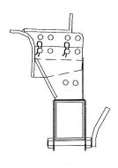
Possible Header Mount positions for Rectangular Frame Headers. The Header Mount can be adjusted up, down, forward or backwards, depending upon the type of header being transported.
