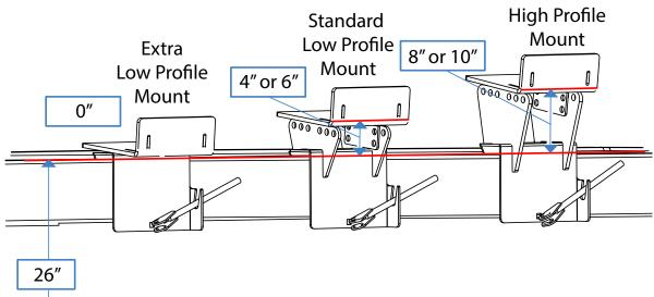
Measurement for "Ground to Top of Bar Height" is based on standard tires and apex of the crown of the bar.
