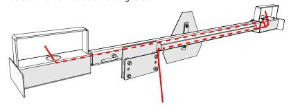
• Plug the lights into the harness and mount them on the light bar using 1-1/2" self-tapping screws. Ensure the red and amber lights are facing to the rear and the amber light is on the outside.
