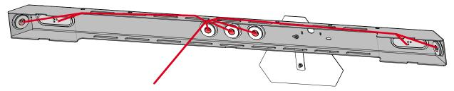
• Connect the stacked four pin of the rear harness to the main harness.
