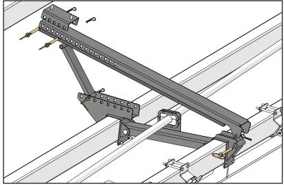
10. Place the upper bar back in place and secure using the 3 upper bar clamps and 1/2"-13 SF hex nuts. Remove the slack in the light wire by threading the excess wire back through the tongue. Secure the excess cord to the cord wrap on the tongue.
