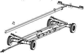
3. Take one side of tie rod off by loosening the 3/4" shoulder bolt nut and removing the 3/4" shoulder bolt. **The shoulder bolt is** threaded part of the way so you must unthread the bolt to remove it.
