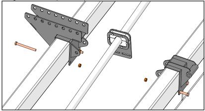
7. Bolt the upper bar center support brace to both support brackets using  $3/4"-10 \times 6"$  hex bolts and 3/4"-10 nylon locking hex nuts. Ensure the center support brace is attached with the holes for the guide blocks facing the rear of the header transport. Tighten the 1/2"-13 hardware shown in the previous step.
