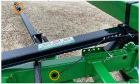
2. Remove the 1/2''-13 SF hex nuts that hold both upper bar clamps. Using a hoist or a fork lift, remove the upper bar.
