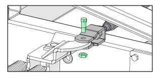
6. Place the upper bar center support brackets on the header transport. The small bracket will straddle the support in the middle of the header transport (as shown below). Place the large bracket on the corresponding bar so they are aligned. Put the 1/2"-13 x 5" hex bolts and 1/2"-13 centerlock hex nuts into place and leaving loose until step 7 is complete.
