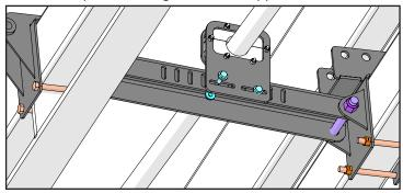
9. Place the lifting arm and upper bar support arm on the center support brackets. Pin the lifting arm and upper bar support arm in the same holes that are used in the front and back of the header transport.
