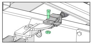
4. Remove the old tie rod support arm. To complete this step, first remove the guide blocks by loosening and removing the 1/4"-20 x 2" hex bolts and 1/4"-20 nylon locking hex nuts that surround the tie rod. The guide blocks and their hardware will be reused later, so set them to the side. Then, loosen and remove the 1/2"-13 x 5" hex bolts and 1/2"-13 centerlock hex nuts. Lower the tie rod and slide off the support arm.
