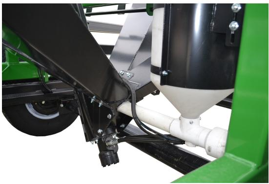
**NOTE:** To turn the speed of the Talc Applicator up or down adjust the knob at the base of the Talc Applicator located directly beneath the auger rest.
