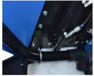
Fasten the Transfer Tube to the Talc Holding Container using the supplied bracket. Start installing the bracket by removing the two bolts shown in the image above. Now fasten the bracket to the door with the two nuts that were just removed. Install the 3/8" x 3" U-bolt. Use (2) 3/8" serrated flange hex nuts and (2) 3/8" lock nuts to fasten the U-bolt to the bracket. Tighten hardware once installed.
