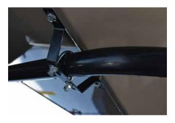
Fasten the Transfer Tube to the Talc Holding Container using the supplied bracket. Two 3/8" clearance holes will need to be drilled into the shell assembly to install the bracket. Use (2) 3/8" x 1" hex bolts and nut to fasten the bracket to the shell assembly. Install the 3/8" x 3" U-bolt. Use (2) 3/8" serrated flange hex nuts and (2) 3/8" lock nuts to fasten the U-bolt to the bracket. Tighten hardware once installed. Step 6.
