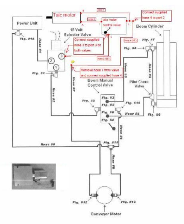
Schematic for Aluminum Selector Valve Only (Not all Seed Tenders are equipped with Selector Valve)
