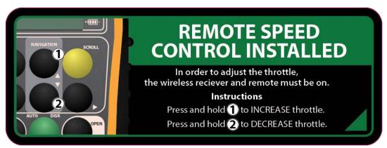
The remote throttle option for the Kar-Tech Wireless System only works with the wireless J&M Mega Remote. This remote and receiver combination provides the output required to drive the throttle control via the 2-wire Deutsch connection. Press the up navigation button on the remote to increase the throttle. Press the down navigation button to decrease the throttle. Both buttons will only be activated when the conveyor is running.
