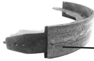
Acceptable Hairline Cracks
