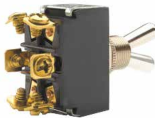
JM0037125 DPDT (On-On) Conveyor Start/Stop (This is a momentary switch, once you let go of the switch it will turn off.)
