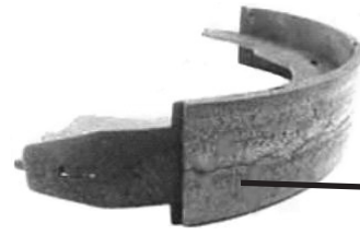
Acceptable Hairline Cracks
