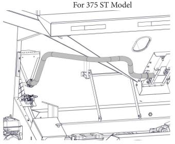
Install the Transfer Tube. Slide the tank end into the Transfer Tube Bracket then push the opposite end into the Talc Holding Container. Using the Exhaust Clamp, tighten the Transfer Tube to the Talc Holding Container. Fasten Hardware once finished.
