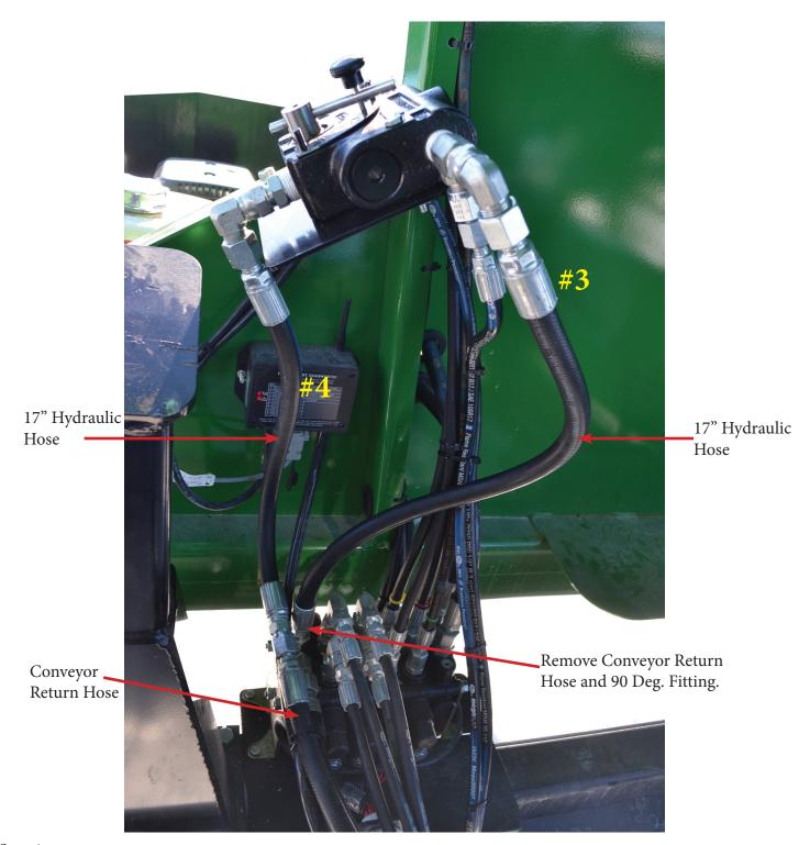
Step 4. Install the last 1/2" x 17" hose. This hose connects to # 4 on the Talc Applicator Valve Body and to the Conveyor Return Hose, which was removed from the Hydraulic Valve Body in step 3. Tighten all fittings once installed.
