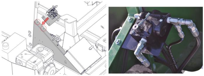
Step 3. On the Hydraulic Spool Valve remove the "Return" hose on the valve body for the conveyor. Install the 1/2" by 17" hydraulic hose from the valve body to the Talc Applicator Control Valve. Connect hose to #3 on the talc applicator valve body. Tighten all fittings once installed.
