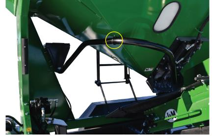
Fasten the Transfer Tube to the Talc Holding Container using the supplied exhaust clamp. Using the black hose clamp and a self tapping screw, fasten the tube to the shell assembly as shown in the image above. Tighten hardware once finished.
