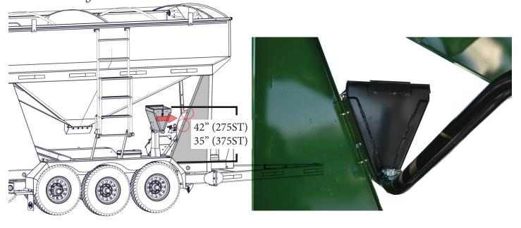
Step 2. Using the Talc Control Valve Body Assembly mark (2) holes in the front left leg gusset. The bracket should be placed at the highest point possible on the front leg gusset. Once marked, drill 2 holes with a 7/16" drill bit. Attach the Control Valve Body Assembly with (2) 3/8" x 1" Serrated Flange Hex Head Nuts and Bolts. Tighten hardware once finished.
