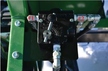
Step 9. Use zip ties to fasten hydraulic hoses where necessary. Hose's should be fastened where they will not rub any moving components or catch any debris during transit.
