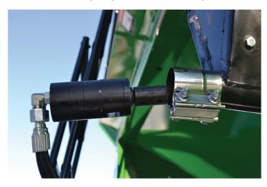
Step 8. Install both 1/4" x 107" Hydraulic Hoses from the Talc Motor to the Talc Control Valve Body. Hose coming from Port A runs to Port 1 and Port B runs to Port 2. Route the hose through the conduit on the frame. Tighten fittings once installed.
