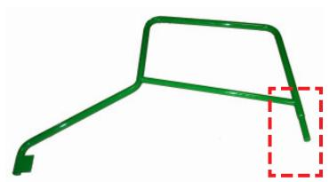
Cut off the lower end of your existing handrail at the location shown.
