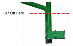
Slide the cut-off section from your old handrail onto the end of the new handrail as shown.
