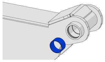
12. Use the bushing kit in the position shown below and tighten the nut to press in the new bushing and replace the seal that was taken out in step 11.
