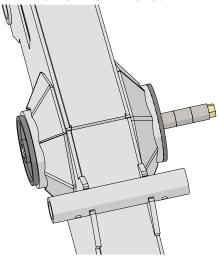
8. Swith sides and repeat the process with your second bushing. When finished with one side be careful not to scrape the inside of the bushing with the bolt.
