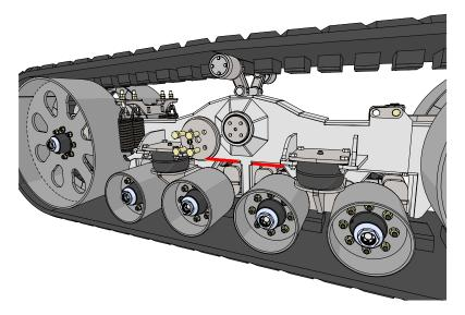
2. Use forks of tractor to lift the belt off of the upper mid-rollers. Take off the upper mid-rollers by removing both 1/2" x 3" bolts and 1/2" nuts shown below.
