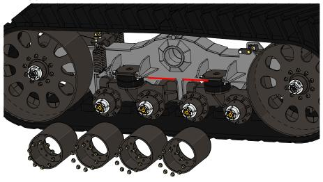
6. now slide the whole weldments out of the side that has the bogies still attached. Spraying WD-40 on the belt will help the hubs and wheels slide more easily against the belt surface.
