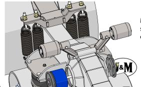
Make sure that this plate is seated evenly on the spool end before tightenting.
