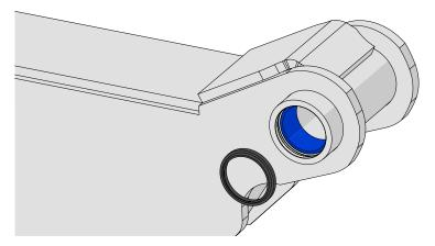
11. Remove the bushings with the help of a dremel tool or something similar. Be careful not to mar the inside of the steel spool.
