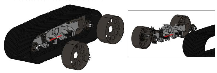
8. Remove the end idler wheel. Remove the  $3/4" \times 5"$  bolt to remove the pin.
