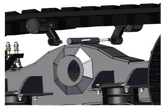
3. Loosen the nuts on the tensioner shown below with 1-1/8" ratchet wrench. For easier removal, place one fork of the forklift near the edge of the tensioner spring plate and maintain downward pressure to relieve pressure sooner from springs. Once nuts have been removed, ease off with the forklift.
