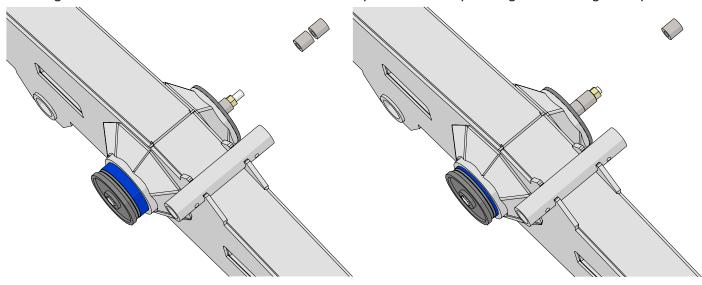
7. The bushing should end there when you tighten the plates until they meet the spools on both sides. **READ STEP 10 IF YOUR TRACKS WERE MADE BEFORE 2019!**
