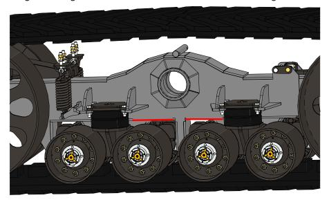
5. Remove the four bogies on the opposite side of the tracks as the forklift. Set the track down and pick it up from the opposite side in the same location.
