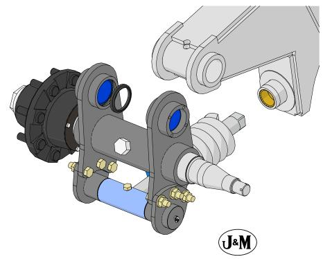
14. Remove the bushings with the help of a dremel tool or something similar. Be careful not to mar the inside of the steel spool.
