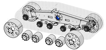
6. Remove the (2)  $3/8'' \times 1-1/2''$  bolts and the tensioner stopping plate.
