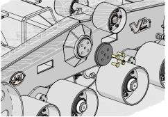
2. Use tractor forks to pull the tracks off of the axle.
