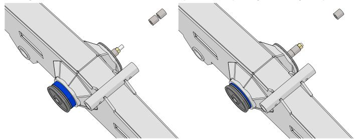
8. The bushing should end there when you tighten the plates until they meet the spools on both sides.
