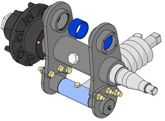
15. Use the bushing kit in the position shown below and tighten the nut to press in the new bushing and replace the seal that was taken out in step 13.
