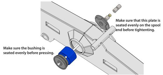
7. As you tighten the nut you will need to hit the opposite side with a dead blow to make sure the nut keeps traveling. You will need to remove the nut and add a spacer to finish pressing the bushing to its place.
