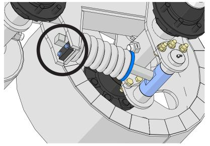
7. Loosen the spring tensioner until it stops using the socket supplied with the tracks (1-5/16" socket).
