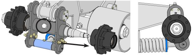
12. Remove the 5/16"-18 x 5/8" bolts and the two end plates and the 3/4" nut shown in green. Pull up on the bottom of the tensioner as shown to let the green bolt drop through. You can the remove the pin that holds the tensioner to the track itself.
