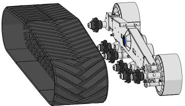
9. Remove the mid-roller center pivot pin by first removing all eight 5/16"-18 x 5/8" bolts and the two end plates. Then remove the 3/4" x 5" bolt in the center and take the pin out.
