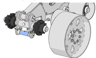
10. Remove the dust cap, spindle pin, the castle nut, and washer.
