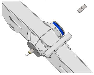
10. If this is the only thing to replace, go through the steps backwards to put your tracks back together. **Be careful** when sliding the track center pivot through with brand new bushings.
