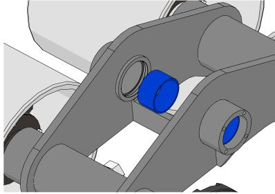
12. Set up the bushing kit as shown. Tighten the 3/4" nut to press in the new bushing.
